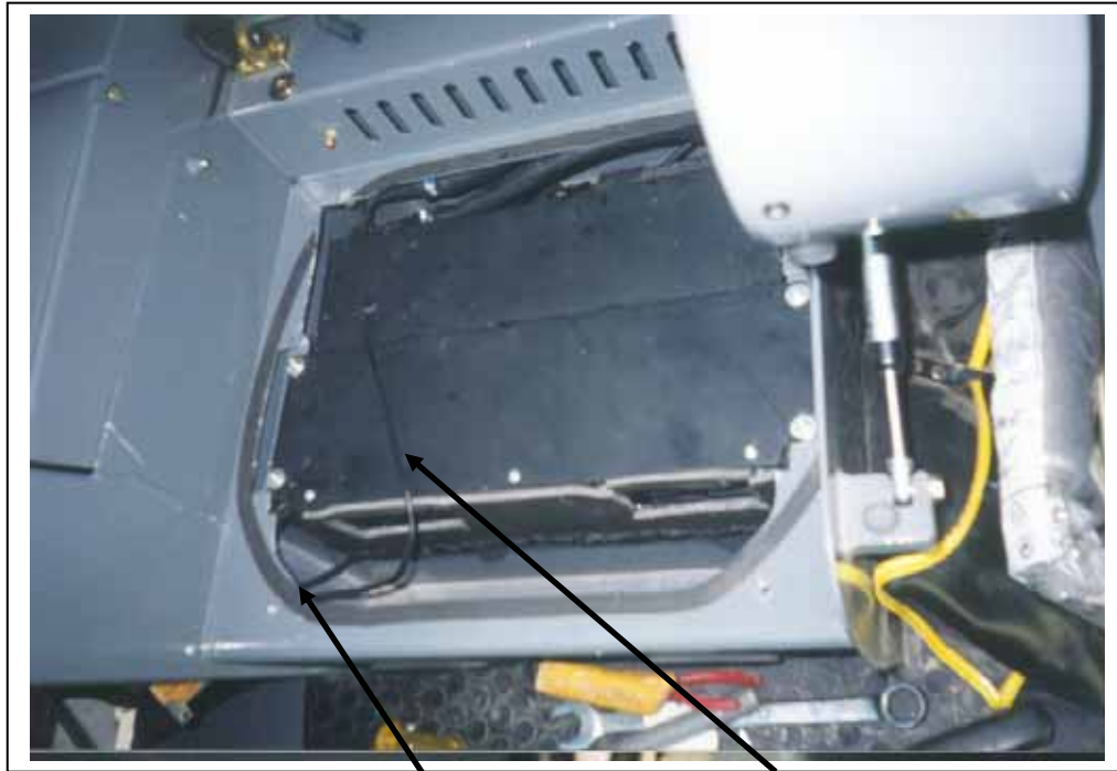
Probe through same hole as heater control cable
