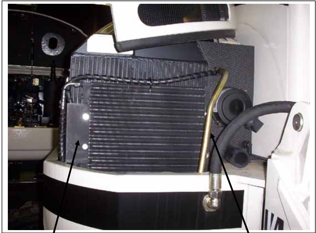
Fitting end bracket
