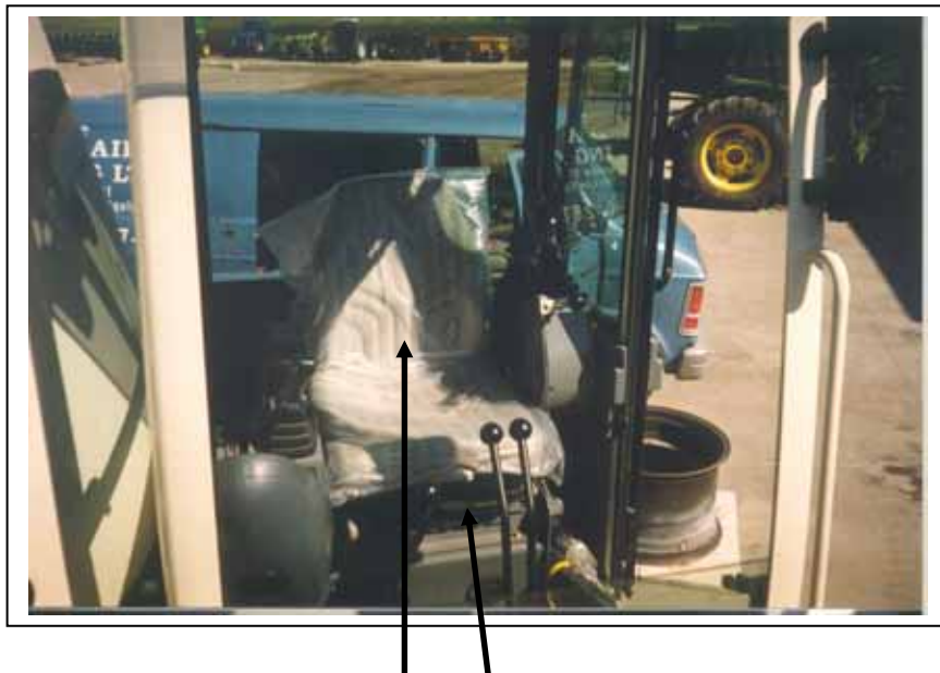
Remove seat and seat frame
