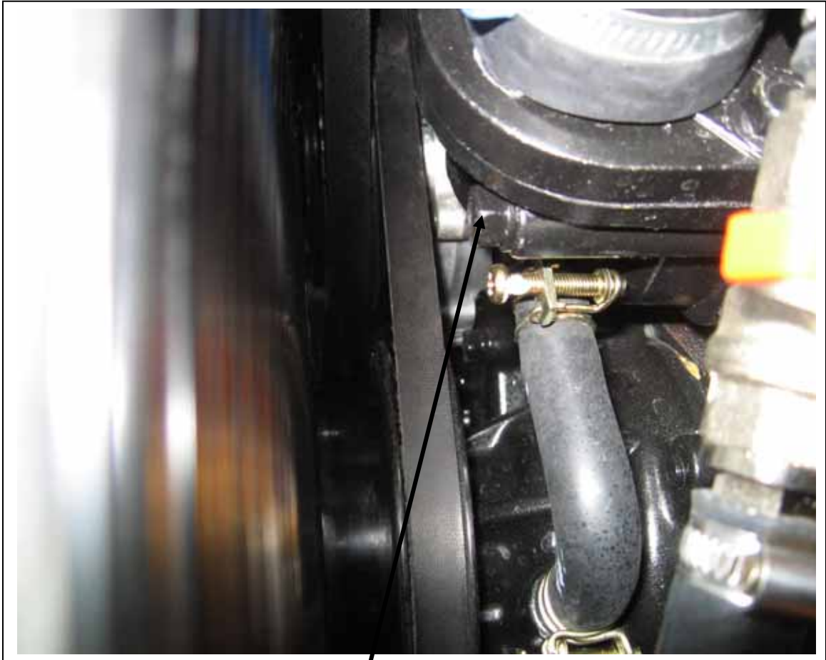
The end of the stiffener bracket with the slot bolts on this point using the ¾” spacer and the long M8 bolt.
