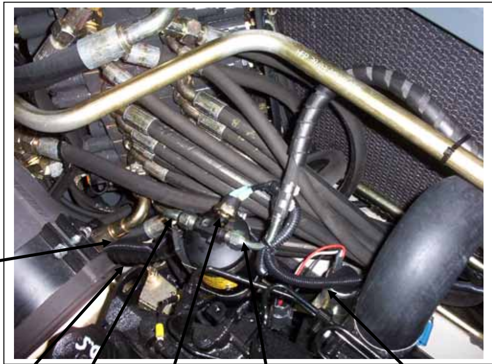
5/16 90° fitting on drier outlet
