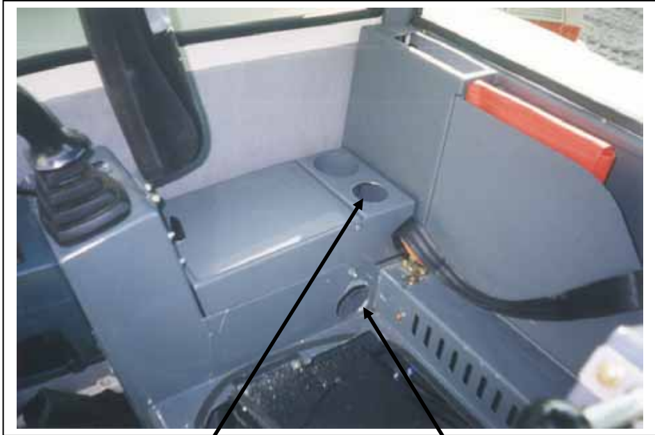
2 ½" hole for snap-in louver
